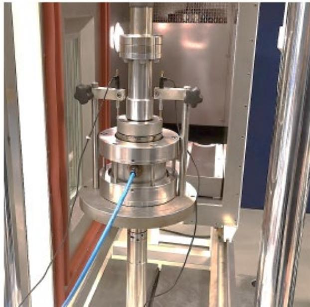
Figure 2: Assembly for Triaxial test
