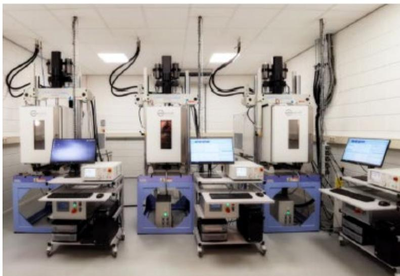
Figure 1: Shimadzu dedicated asphalt testing systems
